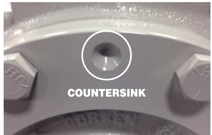
½” drilled countersink on a new pump’s head.
