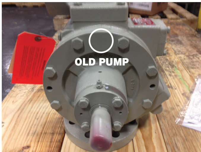
Old pump without the drilled countersink.
